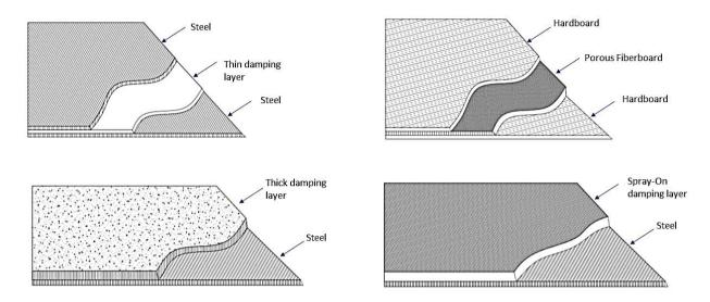
Figure E-25: Cladding of sheet metal and panels
