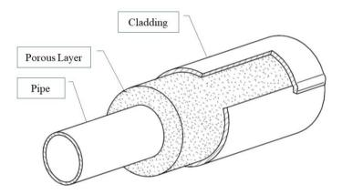
Figure E-24: External lagging for pipes
