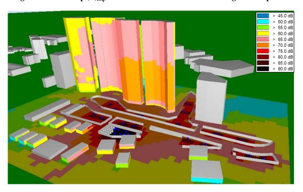
Figure 9: 3-D noise modeling of a construction site located amongst built up areas showing noise levels in the environment and at building facades
