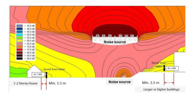
Figure B-4: Microphone position located near buildings or refection surface
