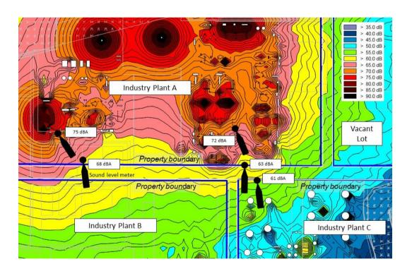
Figure 3: Noise map and suggested measurements at property boundary and sources to determine premise creating high noise
