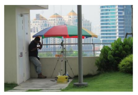
Figure B-16: Example of unacceptable monitoring in progress with sound level meter placed under an umbrella (apparently for weather protection)
