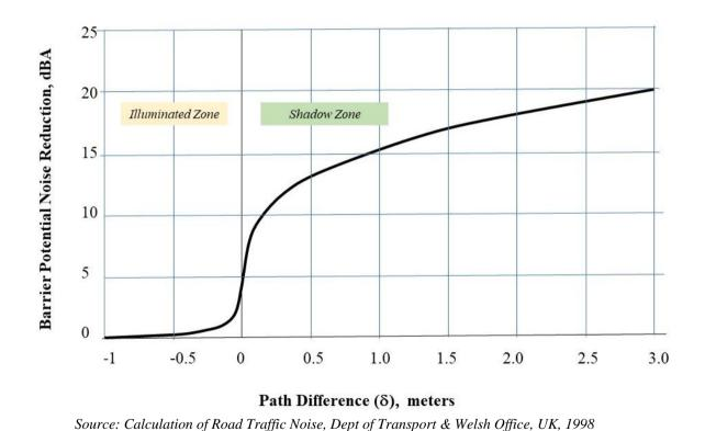
Estimation of barrier attenuation based on path difference
