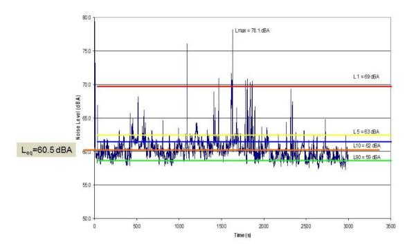
Figure B-24: Noise measurement parameters
