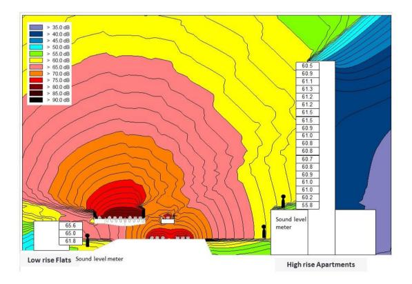
Figure B-6: Noise measurement after project completion
