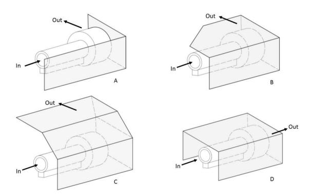
Figure E-17: Examples of different partial enclosures
