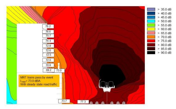
After MRT completion (with MRT trains pass-by)
