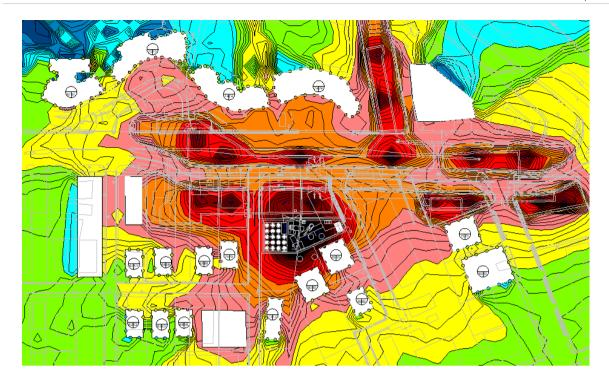
Figure 8: Noise map  $(L_{Aeq})$  for a construction site located amongst built up areas
