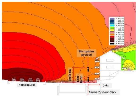
Figure B-3: Recommended noise measurement location
