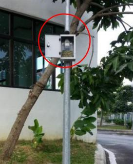
Figure B-15: Examples of unacceptable use of sound level meter installed in a casing as an alternative to permanent noise monitoring units
