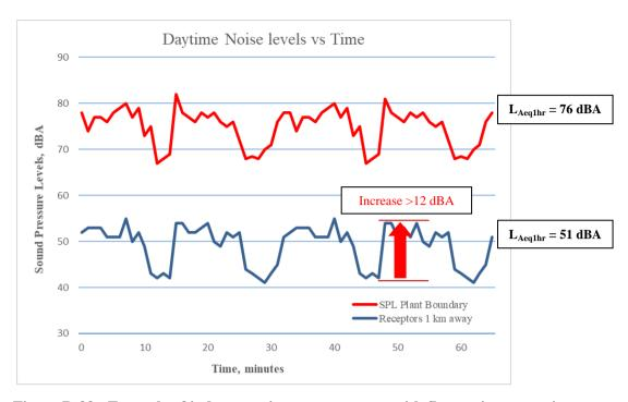
Figure B-33: Example of industry noise measurements with fluctuations over time, measured at plant boundary and receptors
