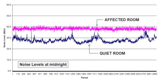
Figure B-45: Instantaneous overall sound pressure levels plotted against time measured indoors in room with line of sight to offending source and another room away from source
