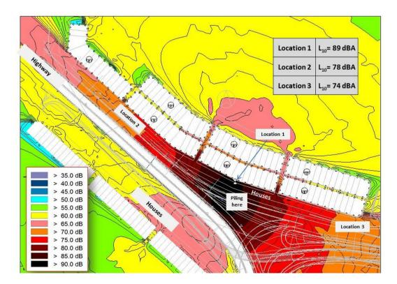
Figure B-35: Example of noise measurements of construction piling (L<sub>10</sub> levels)
