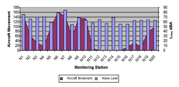
Figure B-41: Example of Daytime  $L_{Aeq}$  for aircraft noise measurement correlated against total number of aircraft movements at 20 monitoring locations
