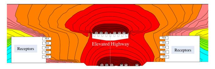
Figure 6: Noise contours ( $L_{Aeq}$  levels) in a cross-sectional plot from 3D noise modelling of an elevated highway superimposed onto existing roads showing noise levels at different floors in multi-storey buildings
