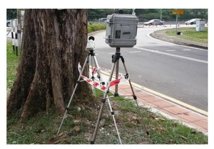
Figure B-17: Example of unacceptable monitoring in progress with sound level meter obstructed by objects (and adjacent extraneous noise source)
