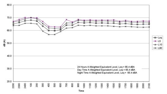
Figure B-43: Example of outdoor entertainment noise measurement results measured at receptors building open terrace (5<sup>th</sup> floor) fronting entertainment outlets.
