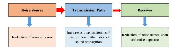
Figure E-1: Basic elements in noise control
