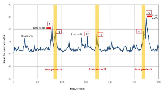
Figure B-28: Noise levels vs time plotted in 1 second intervals over several trains passby events measured in urban environment with road traffic
