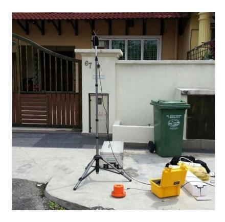
Figure B-1: Example of sound level meter for environmental noise measurements
