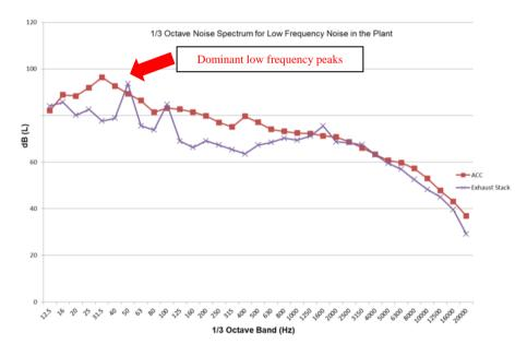
Figure B-34: Example of noise measurements using linear weighting (or Z-weighting) in onethird octave centre frequencies for assessment of low frequency noise
