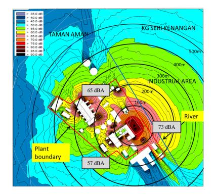
Figure B-32: Example of industry noise propagation to plant boundary and environment adjacent industry premise
