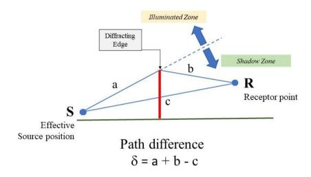
Figure E-3: Path difference for barrier
