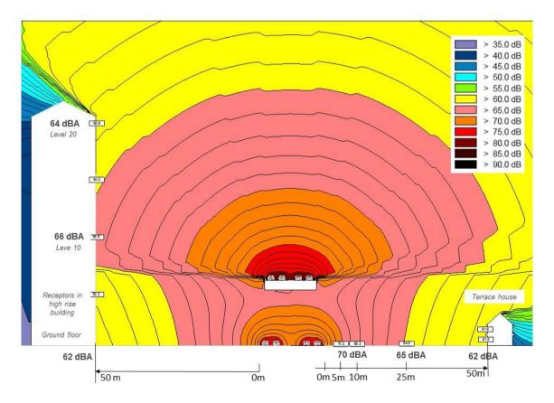
Figure A-4: Noise propagation from line sources (highway) on grade and elevated viaduct to receptor at different distance and elevation to source
