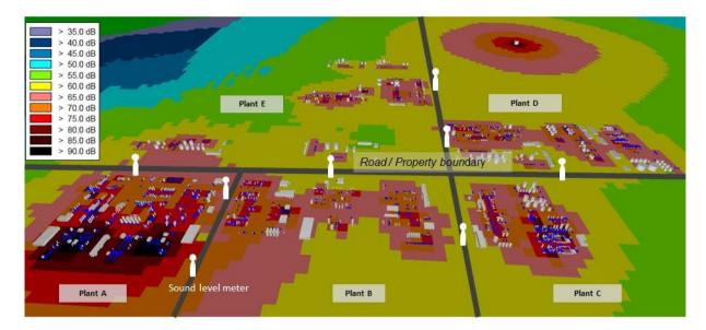
Figure B-7: Example of noise measurement locations at industrial sites
