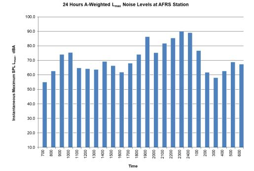
Figure B-40: Example of 24 hours continuous noise measurement of aircraft noise at receptor nearby Airport showing hourly  $L_{max}$  levels
