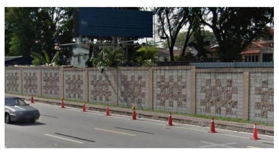
Figure E-8: Masonry noise barriers used in highway noise mitigation
