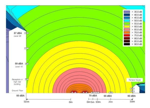
Figure A-3: Noise propagation from line sources (highway) on grade to receptor at different distance and elevation to source
